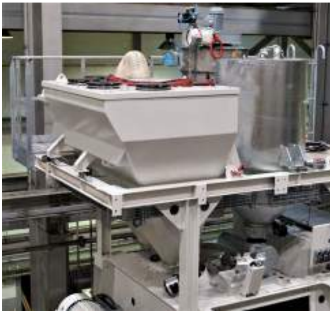
Pre-assembled scales frame with cement and water weigher and dedusting filter.
